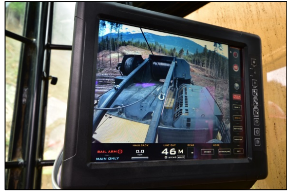
Figure 7. In-cab monitor of drums.
