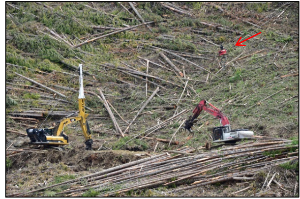
Figure 2. Harvestline, loader and carriage (downhill yarding).
