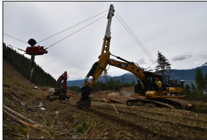
Figure 3. Harvestline set-up location on low side of built road.
