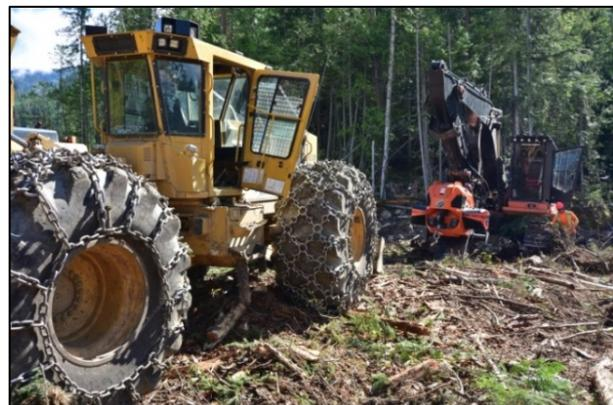
Figure 2. Excavator mounted Traction-Winch T10 with assisted skidder at roadside landing.
