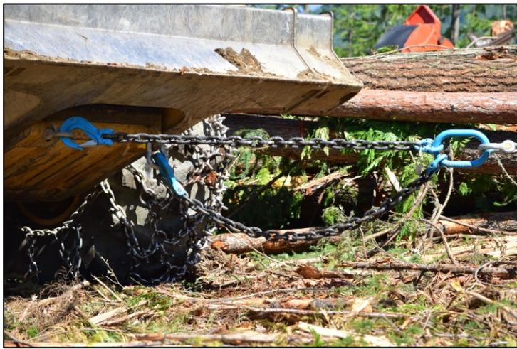
**Figure 4. Mounting points on front of Tigercat 630E grapple skidder.**
