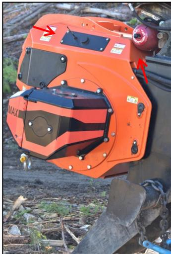
**Figure 5. Traction-Winch (note hydraulic accumulator and communication antennae).**
