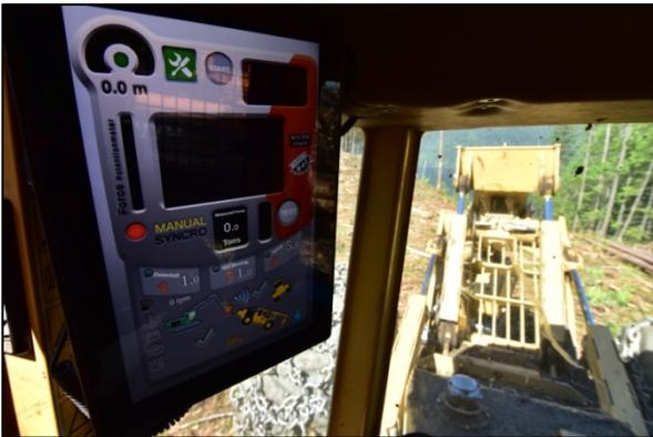
**Figure 7. iWinch Control System monitor mounted inside the skidder cab.**
