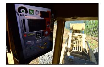
Figure 7. *iWinch Control System* monitor mounted inside the skidder cab.
