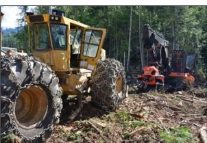
Figure 2. Excavator mounted Traction-Winch T10 with assisted skidder at roadside landing.
