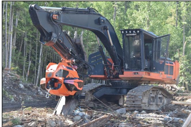
**Figure 3. Hitachi 290 Forester mounted with the TIMBERMAX Traction-Winch T10.**
