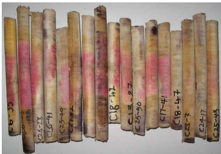
Figure 1 E. bosistoana cores stained with methyl orange. Heartwood is highlighted pink.
