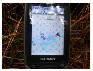
Figure 4. Random GNSS error when static (blue line).
