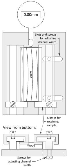
Figure 1. Front and bottom views of Swellometer jig.
