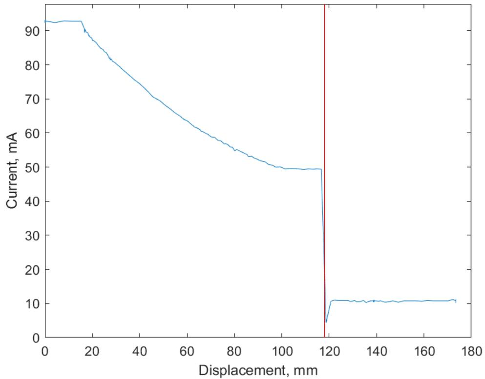
**Fig. 3.** Typical electrical current drop (blue) and switch position determined by the sapwood tool (red) in the tool verification test.
