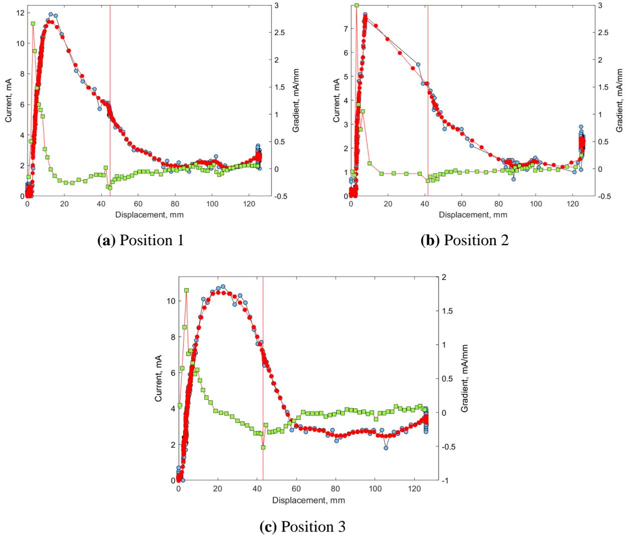
**Fig. 6.** Change of electrical current with displacement within the *E. nitens* log at Positions 1-3. The blue and red circles denote the experimental raw and filtered data respectively. The green squares represent the gradient of electrical current calculated from the filtered data. The vertical red line indicates the SW/HW interface position estimated by the sapwood depth tool.
