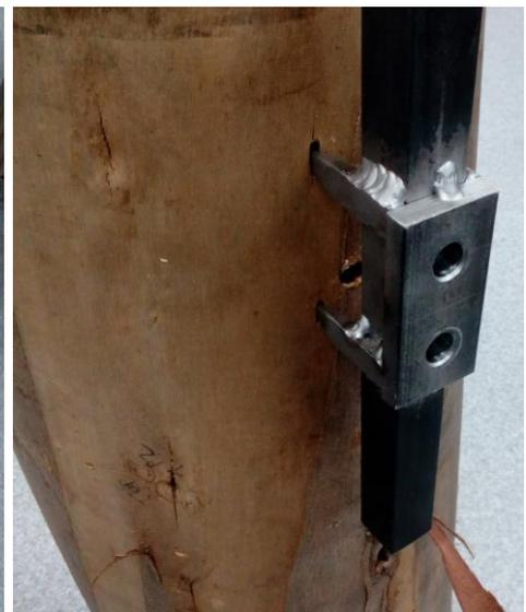
**Fig 5.** Drill stencil in position
