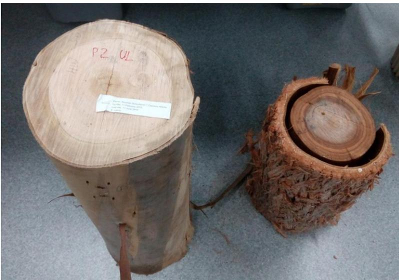
**Fig. 4.** *E. nitens* (left) and *E. globoidea* (right) test logs.
