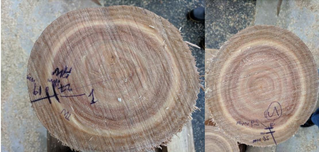
**Fig. 8.** Two typical cross-cut views of *E. globoidea* with the distinguishable sapwood, transitional, and heartwood zones.
