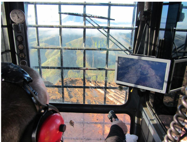
Fig. 3 Cutover camera showing a cable yarder operator a view of trees to be extracted [source: Applied Teleoperation Limited]
