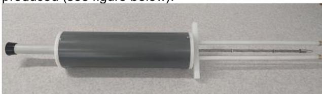
This is used to determine where the boundary of the sapwood and heartwood occurs and hence the proportion of desired heartwood within a tree. Figure below shows the electrical current and current gradient against radial position in the stem of *E. nitens* sample. The vertical redline shows the measured heartwood position. If the tool can be commercialised then field measures of heartwood % will be much faster.
