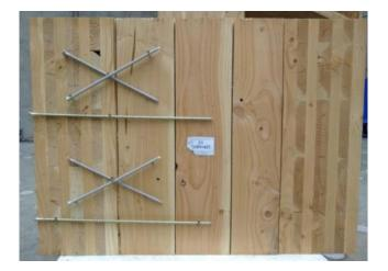
It was found that mixed angle screwed connections showed significant displacement capacity, high strength and stiffness and are suitable for seismic design of CLT buildings with moderate or high ductility in New Zealand. The experimental testing results provided strong technical evidence that the CLT core-walls can provide more efficient lateral load resisting systems for mid-rise and high-rise timber buildings.
