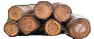
The dynamic stiffness of the *E. bosistoana* veneers averaged 16.6 GPa. One of the *E. quadrangulata* logs did show heart and veneer splitting (shown in the bottom right of the images below).
