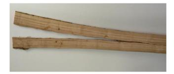
Heartwood quantity and quality were measured in *E. bosistoana*. The data is being used to identify superior families which are now in commercial propagation via both, grafting into seed orchards as well as clonal propagation from coppice shoots of mother plants. Figure below shows bark to bark cores from a number of trees showing the variation in heartwood size (stained pink).
