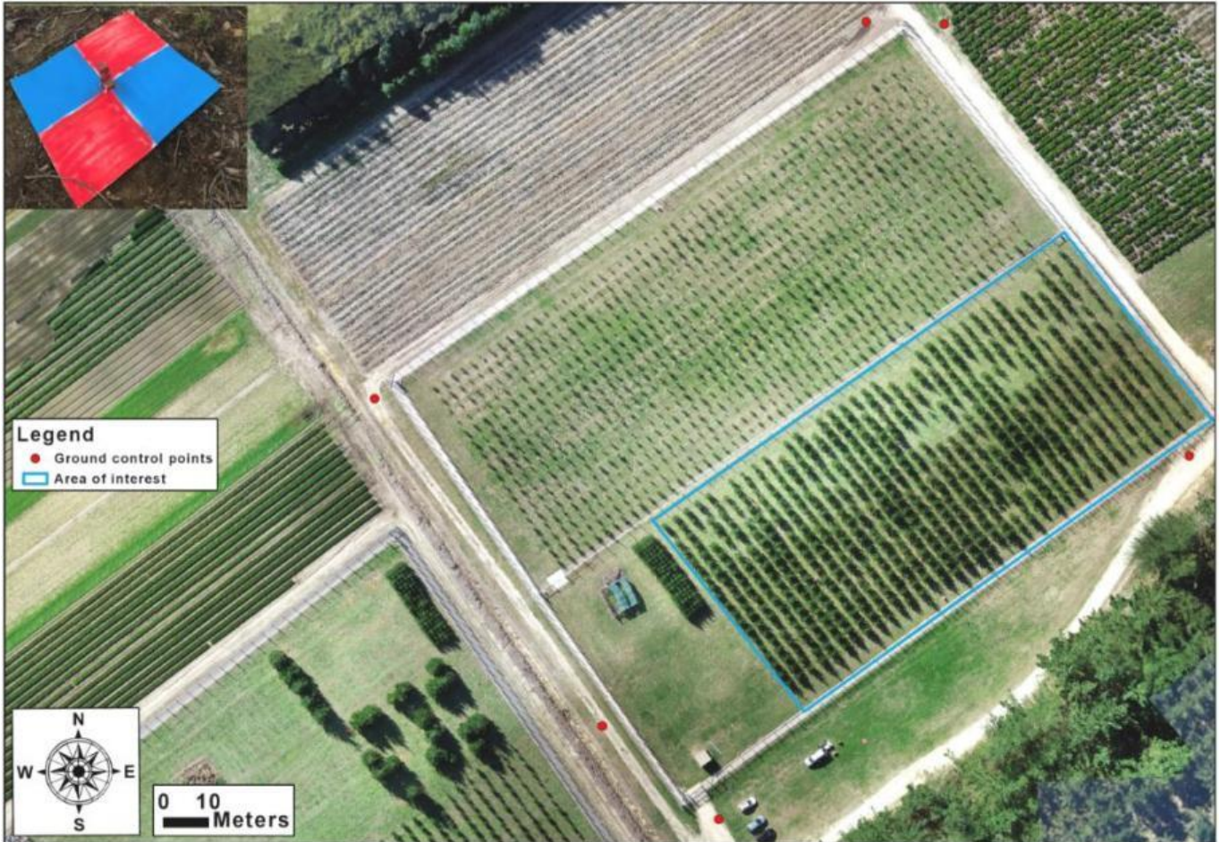
Figure 2. Map of the study site, the area of interest (blue box) and the layout of GCPs across the site, along with an example of a typical GCP marker, as deployed in this trial (inlaid top left).
