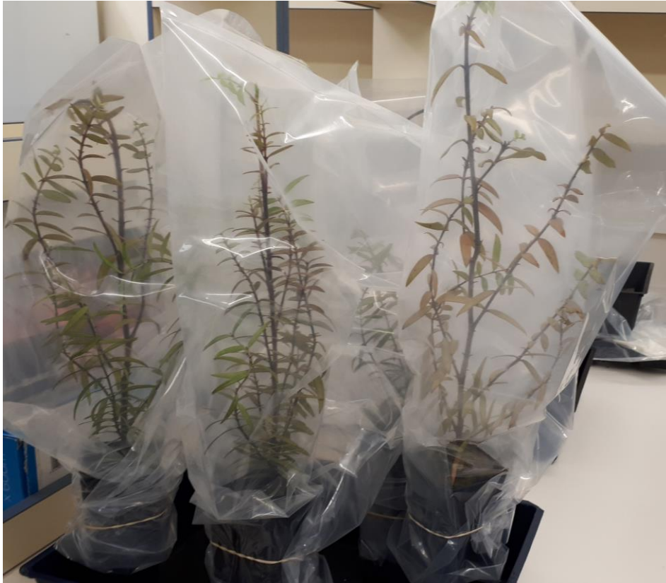
Figure 7: Static enclosures created for collection of VOC emissions from control and inoculated Agathis australis plants.
