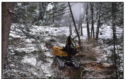
Figure 30. Tigercat LX870D packing a stem to the bottom of the corridor at Case Study 5
