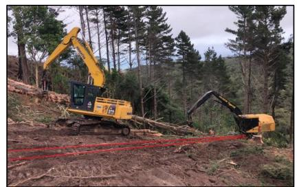
Figure 14. Komatsu PC270 assisting Tigercat LS855C with shovel extraction (winch wire rope highlighted in red).
