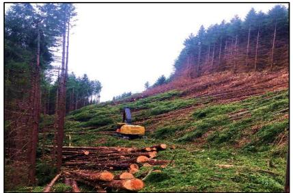
Figure 3. Shovelling along a skid trail (Note: feller-buncher not attached to anchor machine).
