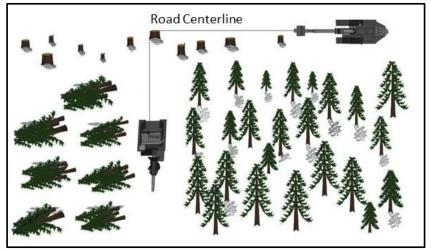
Figure 38. Illustration of operation of a catch tree
