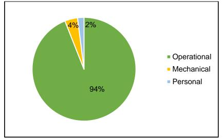
Figure 33. Breakdown of delays recorded by time study at Case Study 6
