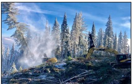
Figure 24. Tigercat L870C and EMS traction line working at Case Study 4 (note snow fall above Tigercat L870C)
