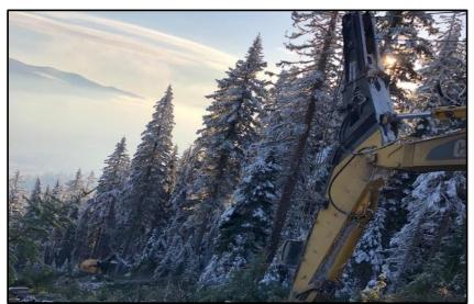
Figure 22. Tigercat L870C felling a stem at the end of a 45 metre corridor at Case Study 4
