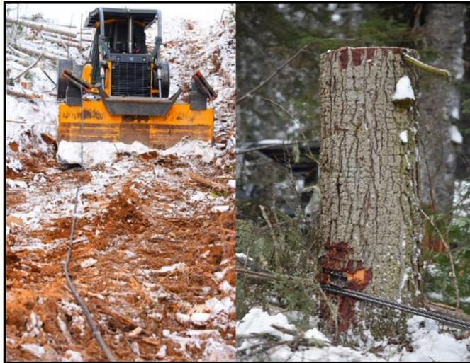
**Figure 37. Example of a catch tree being used at Case Study 6**
