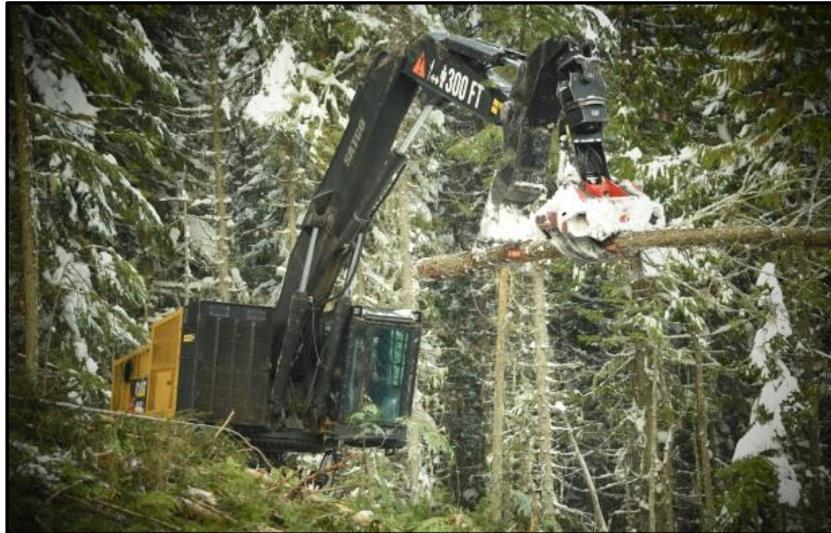
**Figure 35. Cat 552 applying the heel while shovelling**
