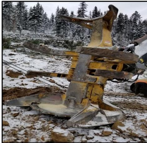
***Figure 25. Tigercat 5702 continuous rotating hot saw***
