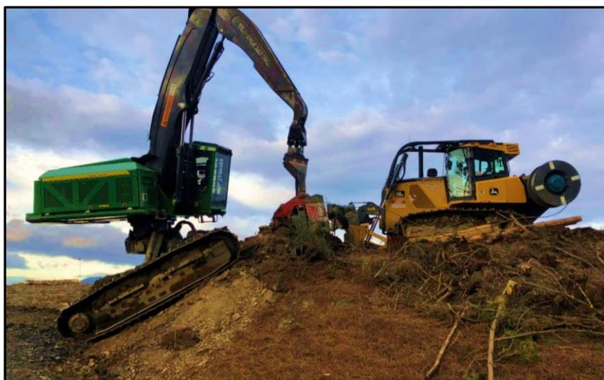
**Figure 6. ROB winch-assist and John Deere 909MH: Case Study 2**
