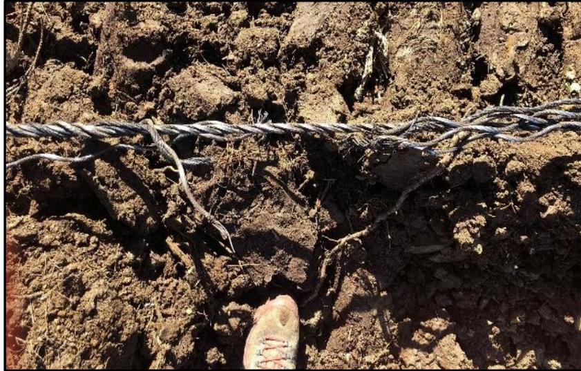
***Figure 18. Wire rope fatigue at Case Study 3 caused from repetitive use on steep slopes and rocky outcrops.***
