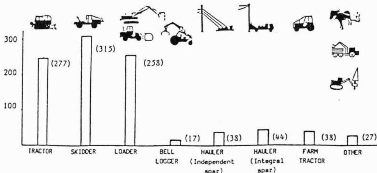
Figure 1: Total number of machines used by New Zealand logging crews, by type (Liley 1985).
