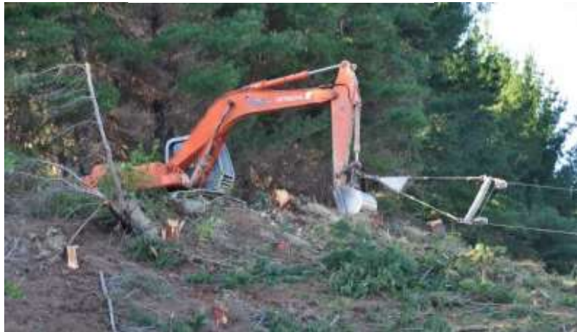
Figure 4: Mobile tail hold machine for CAB system
