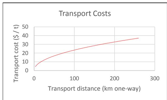
Figure 3: Effect of cartage distance on transport costs
