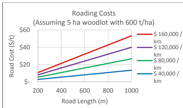
**Figure 2: Roading costs can be significant for small woodlots**
