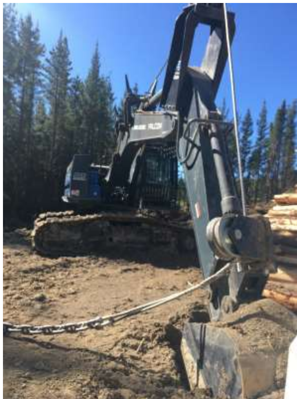
Figure 3. Winch assist machines: a good example of innovation in technology, but overall utilisation has remained relatively low.
