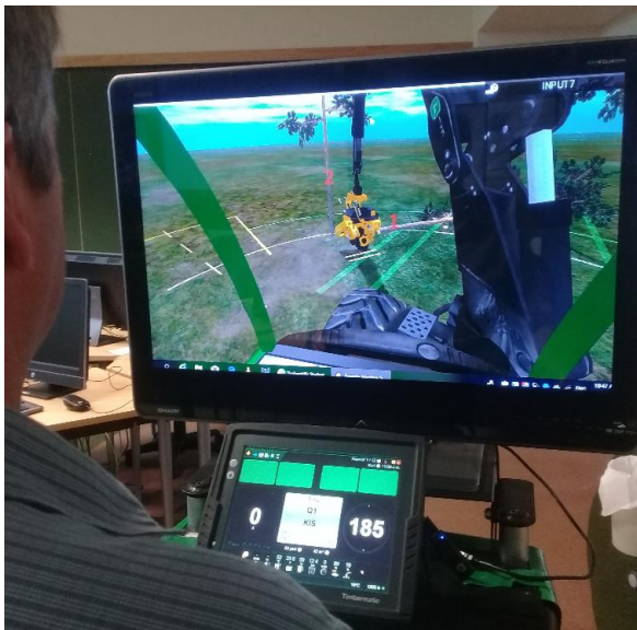
Figure 9: Using TimberSkills training package on the John Deere Cut To Length simulator
