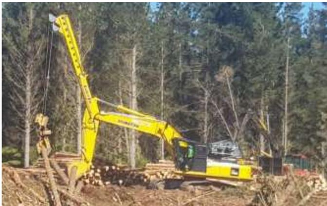
FGR has signed a Letter of Intent with Alpine Logging Equipment Ltd to develop a prototype automated yarding system (using the Alpine Shovel Yarder and Alpine Grapple Carriage) as part of the new PGP programme.
