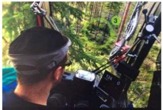
Figure 6: Harvester operator using a head-up display to access information
