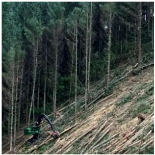
Figure 1: Feller buncher on steep terrain
