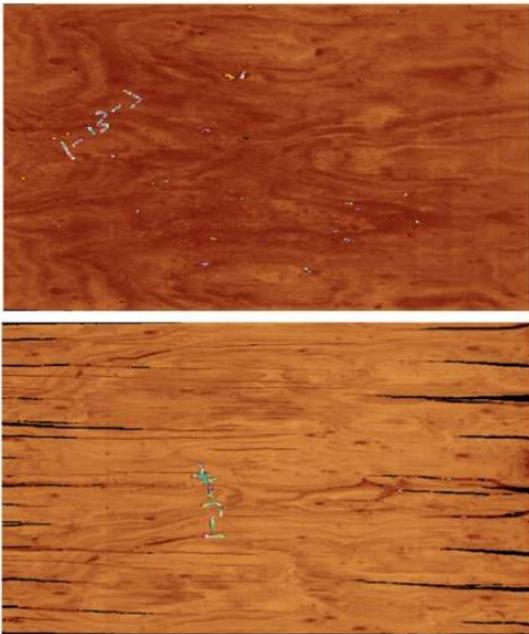
Glue bond trials were undertaken on young *E. bosistoana* and *E. quadrangulata* peeled at NPI. Results indicate that the standard phenolic resins used to bond radiata pine are likely to need to be modified to bond the *E. bosistoana* and *E. quadrangulata* veneer. Image below shows the veneer sheets that were supplied for the testing.
