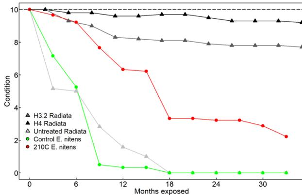
Figure: Fungus cellular stakelet results following 33 months of exposure. A condition of 10 indicates no sign of decay, and 0 indicates complete failure from decay.
