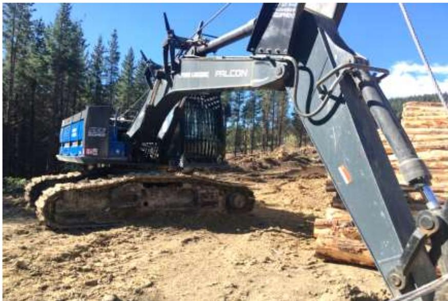
*Figure 6: Falcon Winch Assist machine*
