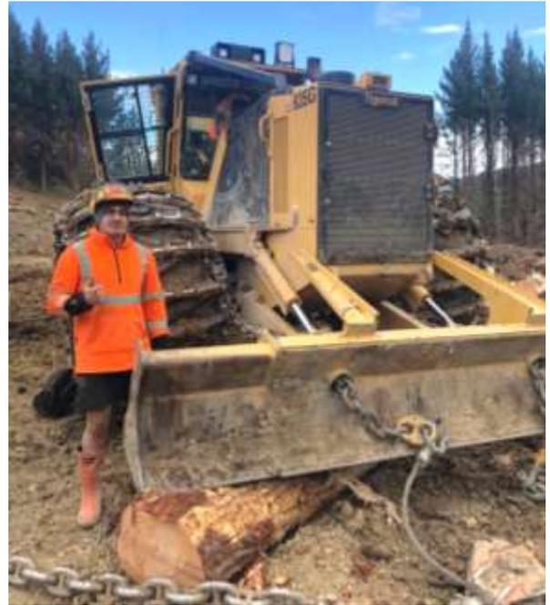
**Figure 3: The Tigercat 635G and Speirs Logging's skidder operator**
