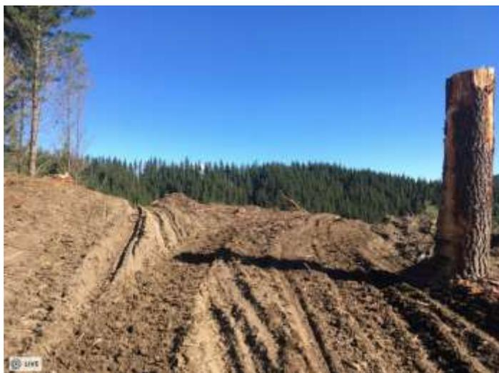
*Figure 24: Tall binding stump used to redirect the rope.*
