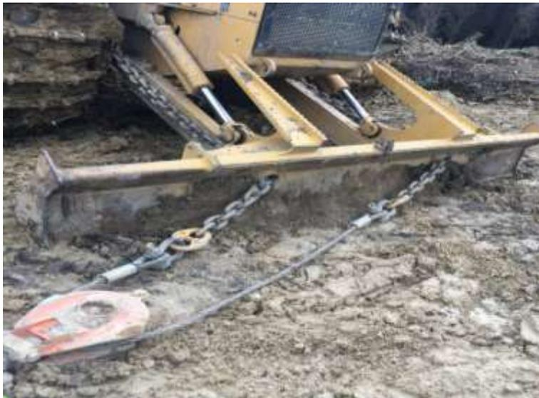
*Figure 5: Attachment method of winch wire rope to skidder*
