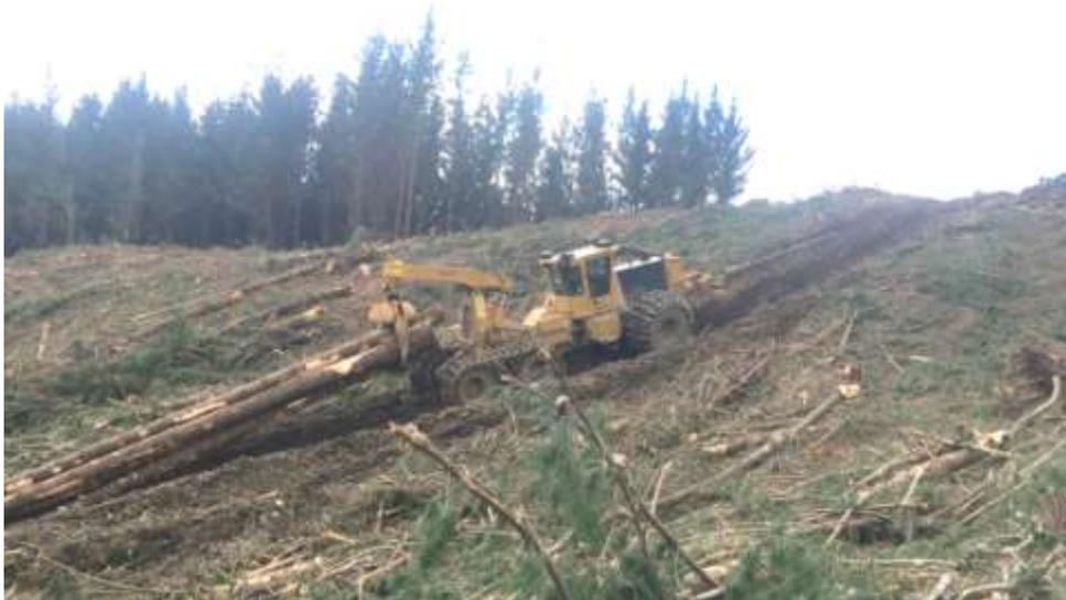
**Figure 2: Tigercat 635 skidder navigating a 30 degree (60%) slope, fitted with a GPS unit to track its location, speed and change in altitude.**
