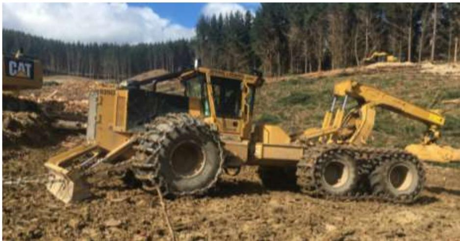
**Figure 4: Tigercat 635 Skidder with chains and belt drive**
