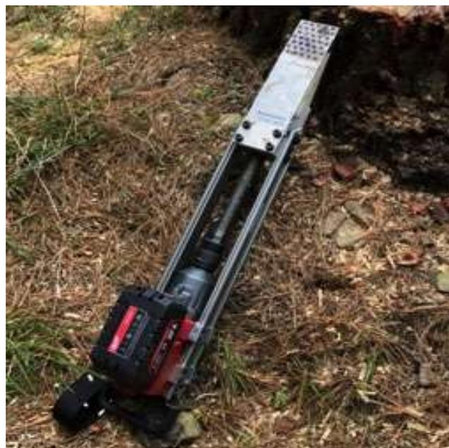
**Figure 3: The TR300 Remote Controlled Felling Wedge**
