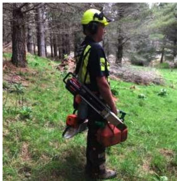
**Figure 8: The TR300 along with all of the other felling equipment could be carried by one person**
