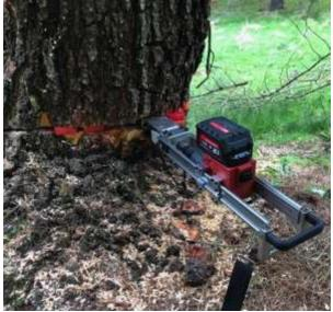
Figure 7: The battery ran flat with the TR300 almost fully extended
