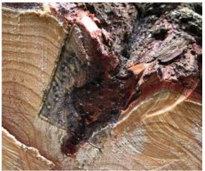
Figure 6: Photo of the bark pocket that affected the lifting capability of the TR300
