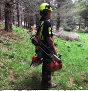
Figure 8: The TR300 along with all of the other felling equipment could be carried by one person
