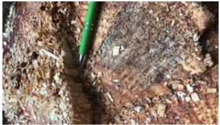
Figure 4: The lip in the slot that pushed the TR300 out of the back cut
