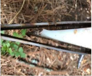
Figure 5: Minor damage to the TR300 wedge
