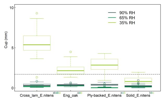
**Figure 3.** Levels of cup at each moisture content for each board type. Superscript letters indicate groups that are not significantly different to each other (95% confidence level) the text colour of the letters indicates the humidity condition they apply to (as per the figure legend). The dotted line indicates the maximum level of cupping allowed by AS 2796 *at the time of installation*.
