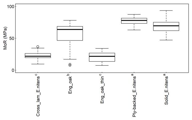
Figure 11. Modulus of rupture (MOR) of different flooring types. Superscript letters indicate treatments that are not significantly different (95% confidence level).
