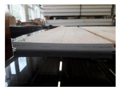
Figure 7. Delamination in an engineered oak board during water soaking
