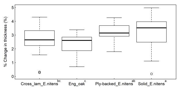
**Figure 2.** Change in thickness between 35 and 90% RH conditions for each board type. Superscript letters indicate groups that are not significantly different to each other (95% confidence level)
