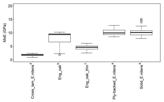
**Figure 9.** Modulus of elasticity (MOE) of different flooring types. Superscript letters indicate treatments that are not significantly different (95% confidence level).
