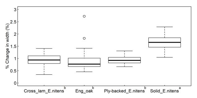
**Figure 1.** Change in width between 35 and 90% RH conditions for each board type. Superscript letters indicate groups that are not significantly different to each other (95% confidence level)
