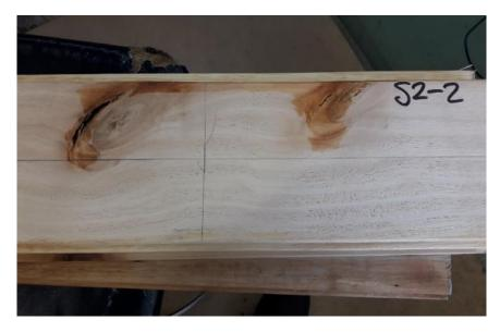
**Figure 6.** Water wicking through a knot to the top face of a solid *E. nitens* board after the lower face was submerged in water
