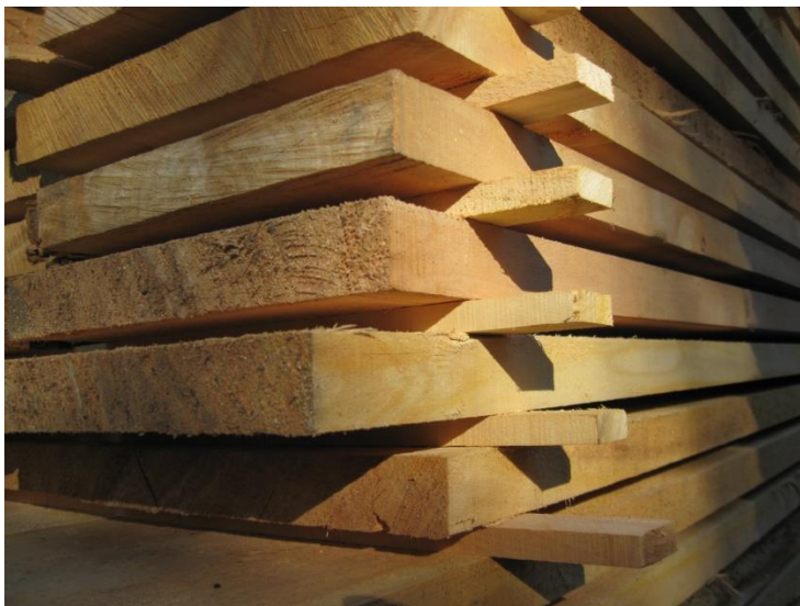
Fig 3: Macrocarpa boards fillet stacked for drying.
