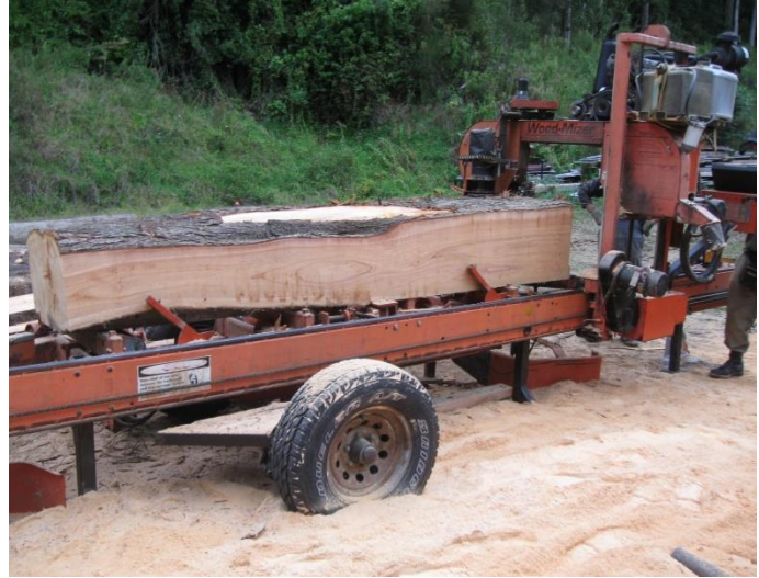
Photo: A large pruned macrocarpa log being sawn with a Wood-Mizer.
