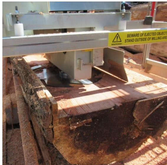
Photo: The swing blade circular saw in horizontal cutting position.
