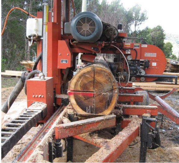
Photo: A Wood-Mizer band sawmill in action quartering a pruned blackwood log.
