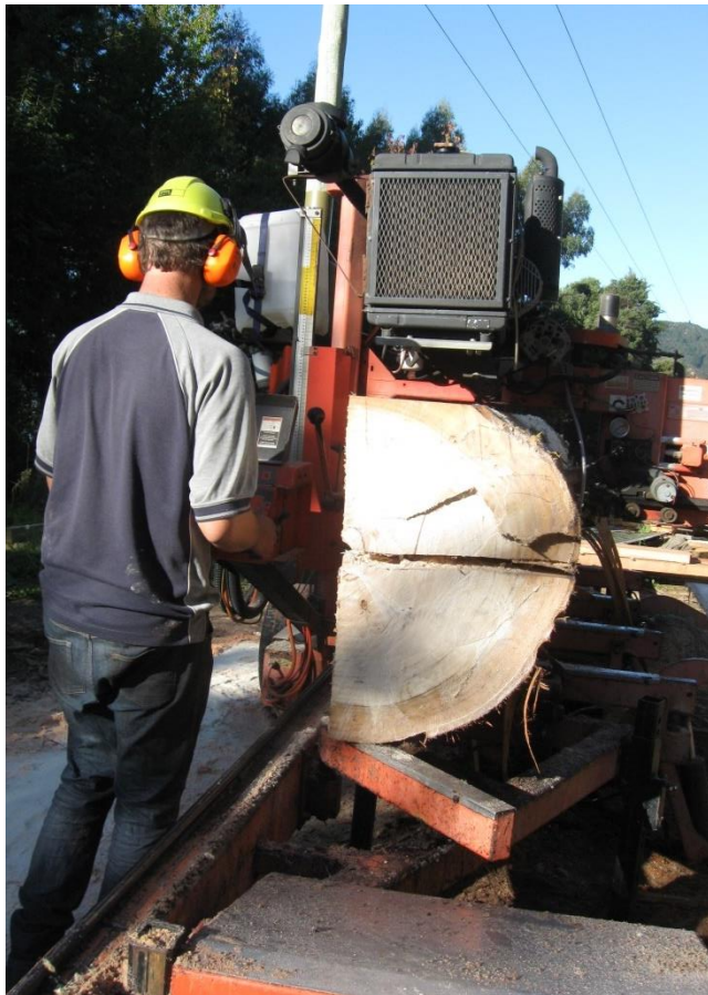
Fig 1: Justin Wells (Logs2Lumber) band sawing E. fastigata pruned log grown at Tai Tane Forest.
