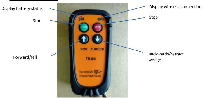
**Information:** The display of the wireless connection flashes regularly to indicate the correct connection. In case of an error, the LED flashes continuously.
