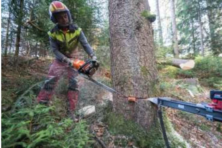
Inserting the release cut of a split level back cut
