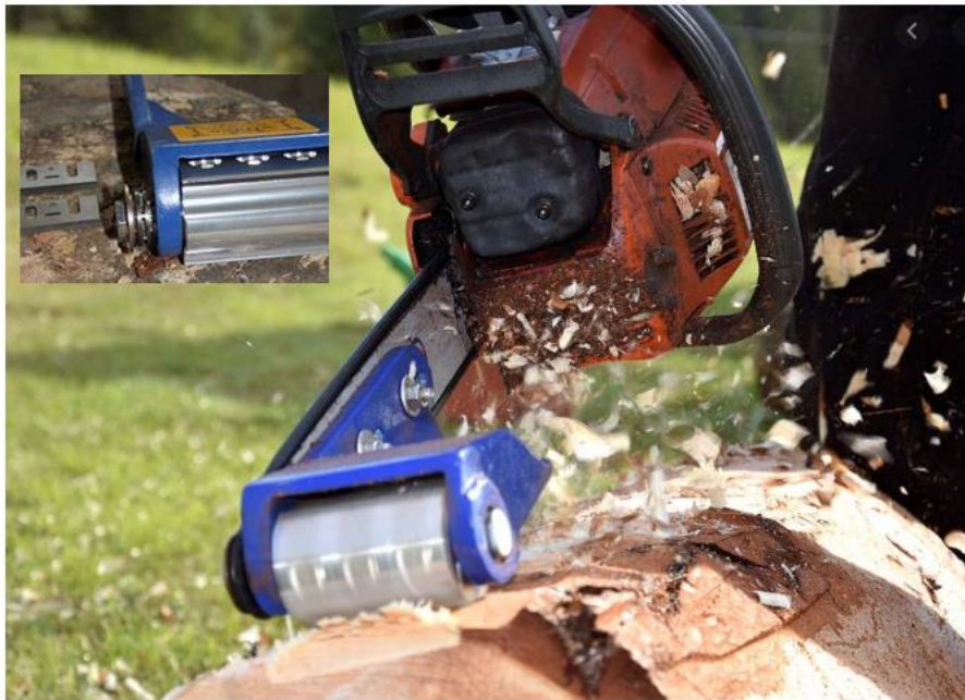
Figure 9. Removing bark with a chainsaw-mounted debarking attachment. The attachment is fitted with two planer blades on a rotating cylinder.
