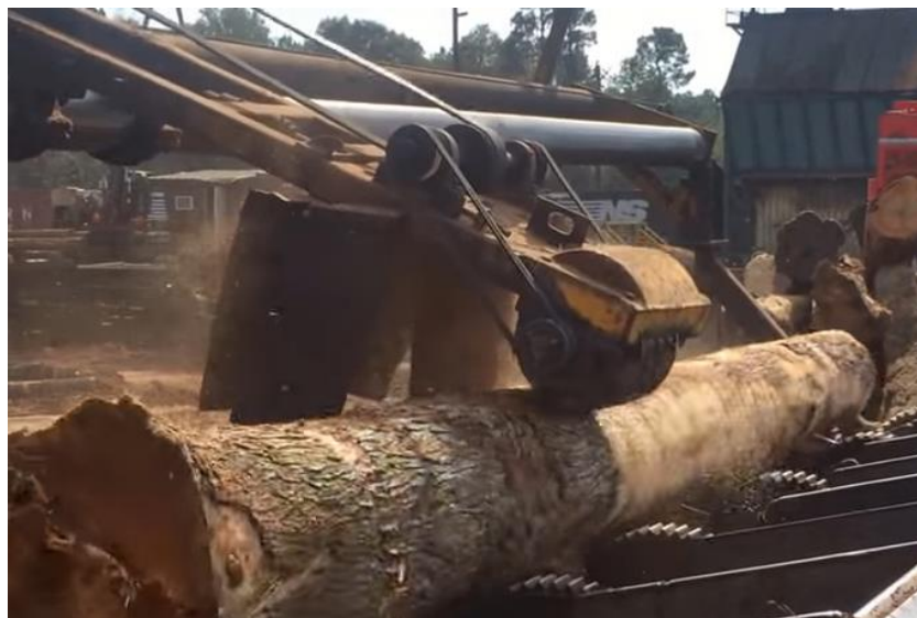
Figure 16. Rosser-head debarker installed in a mill yard. Source: Fulghum Industries Inc.
