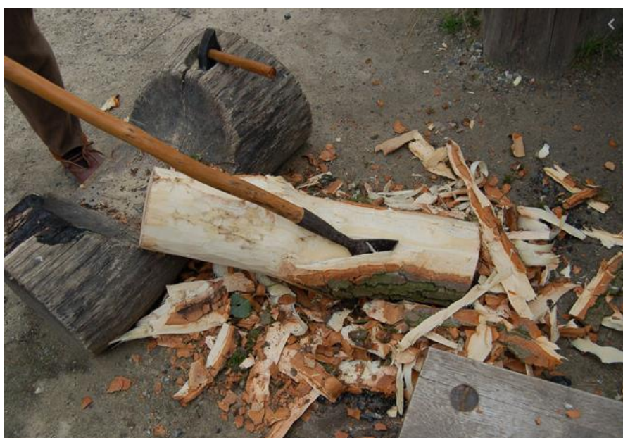
Figure 8. Removing pine bark with a debarking spud allows a less strenuous working posture than using a hatchet or axe.
