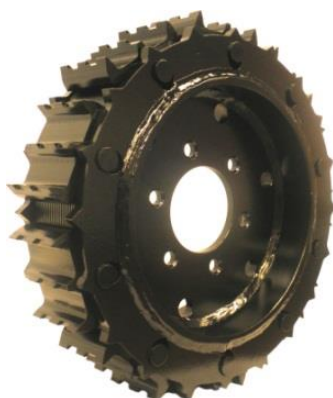
Figure 25. Moipu outer feed rollers manufactured by Moisio Oy in Central Finland. Similar rollers were included in the Australian radiata pine debarking trial.
