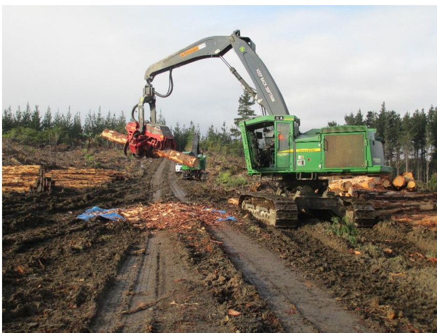
Figure 27. John Deere 909 carrier with Waratah 625c processing head was used in the 2017 radiata pine debarking trial.
