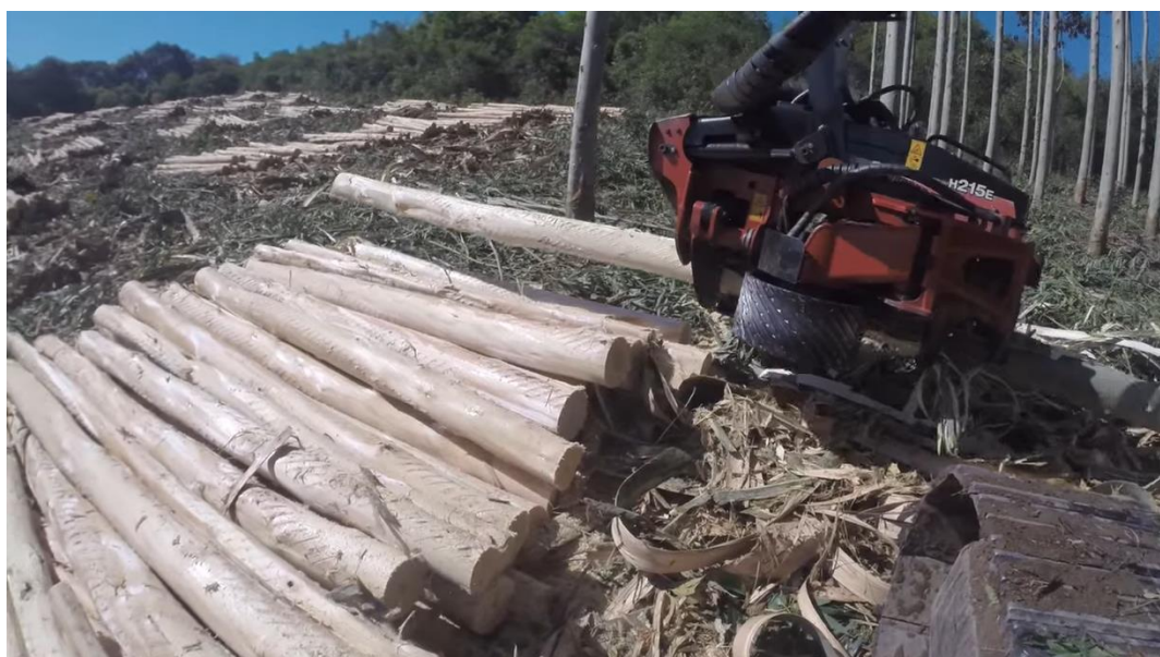
Figure 18. Eucalyptus debarking head being used in a Brazilian plantation.
