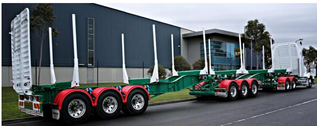
Figure 5. Example of a rear guard on a log trailer and front guard behind the truck cab to contain the load and block any log slippage.
