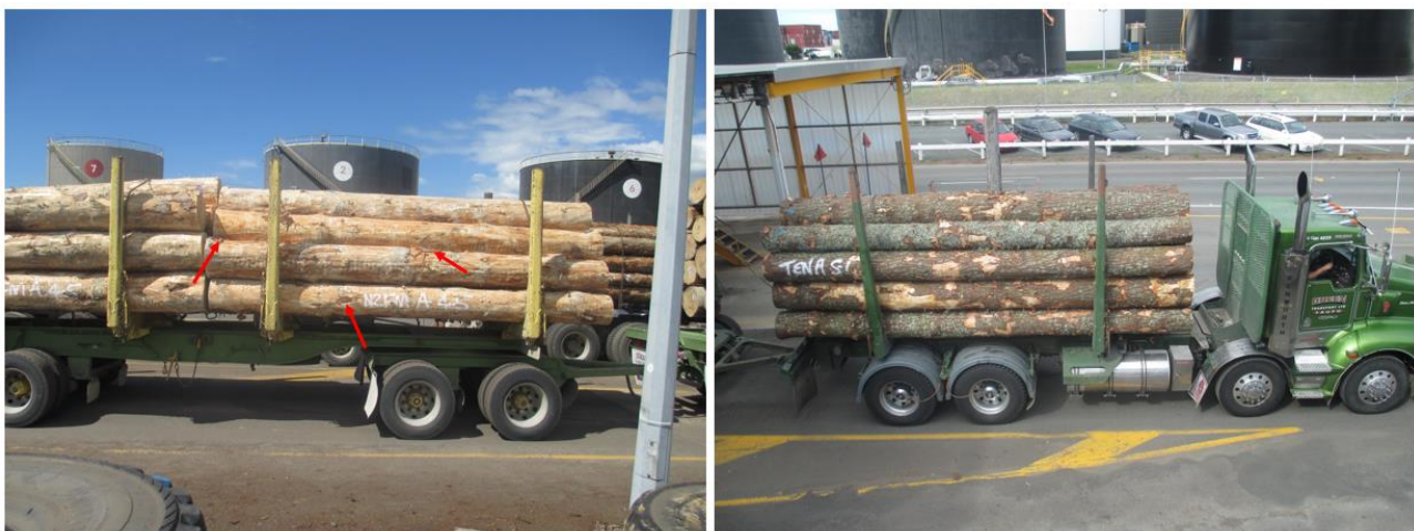
Figure 6. Variation in bark removal from truck loads delivered to the same customer on the same day. Almost all bark had been removed from logs on the left (red arrows point to a few patches of remaining bark). Very little bark had been removed from logs on the right.
