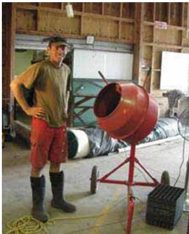
Concrete mixer used to coat P. radiata seed at PF Olsen Nursery
