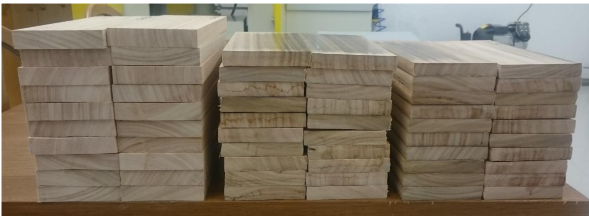
Figure 1: E. fastigata boards following densification. From left to right: undensified controls; surface densification; bulk densification.
