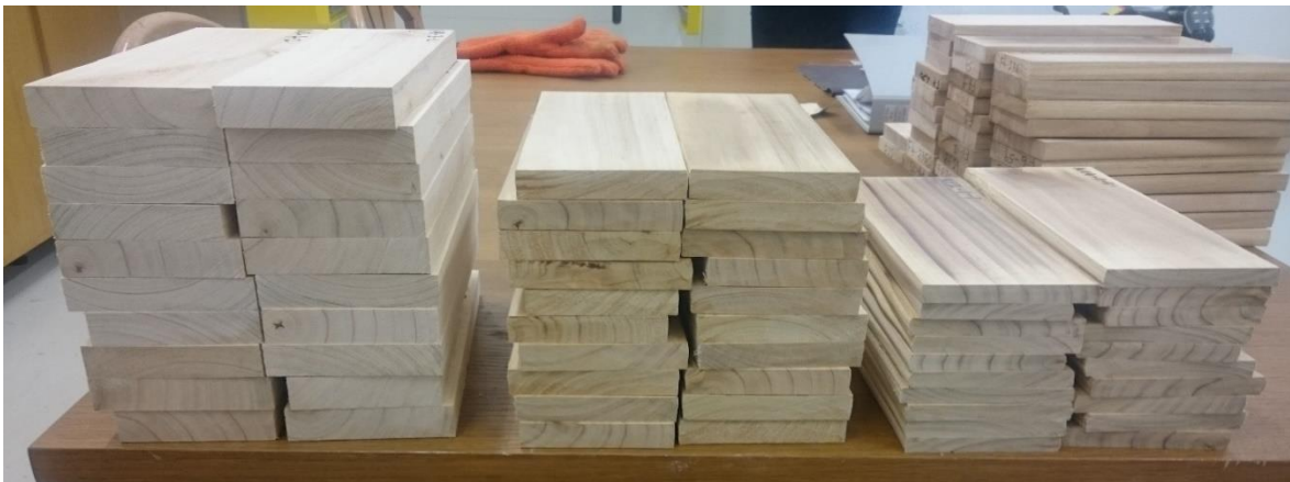
Figure 2: E. nitens boards following densification. From left to right: undensified controls; surface densification; bulk densification.
