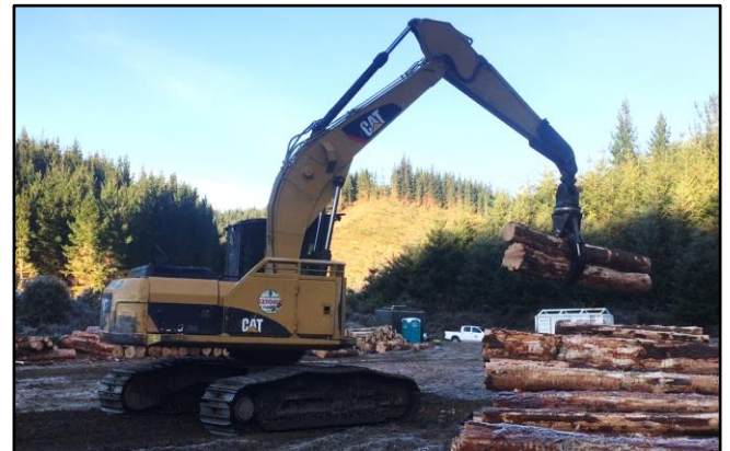
Figure 1: Excavator based loader fleet logs
