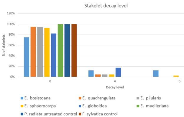
In the in-ground stakes test most of the samples showed a range of minor but established decay through to extensive established and deepening decay. The figure below shows the two untreated controls having 100% failure and the 6 eucalypt species having decay levels mainly 6 to 8.
