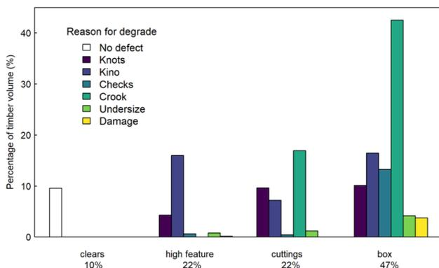
If crook were ignored (assuming it could be removed by improving the sawing process) 19% of boards achieved clears grade, 55% high feature grade and 8% cuttings grade. Overall, this shows that sawing and drying pruned *E. fastigata* is possible, but the sawing methods could be improved to increase overall recovery and to mitigate the effects of crook.
