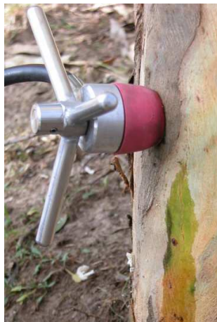
Figure 5. Stemject injector nozzle sealed into injection hole.
