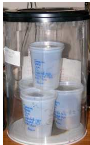
Figure 3. Double containment system used for all Uraba lugens bioassays.
