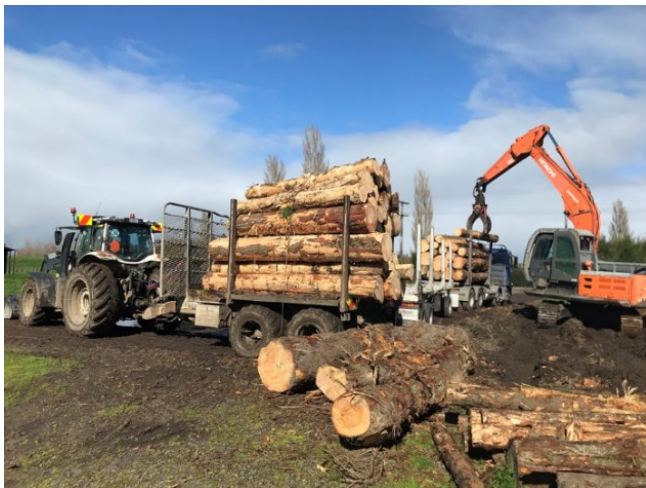
Figure 3: Unloading the forwarder with the Hitachi excavator.
