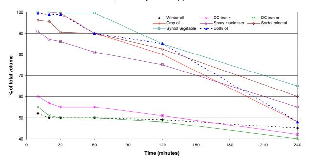
Figure 10. Du Pont, GX569 Copper hydroxide test for eight different spray oils over time.
