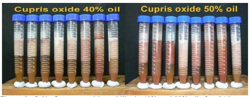
Figure 3a & 3b. Cuprous oxide stability in 40% and 50% oil after 24 hours.
