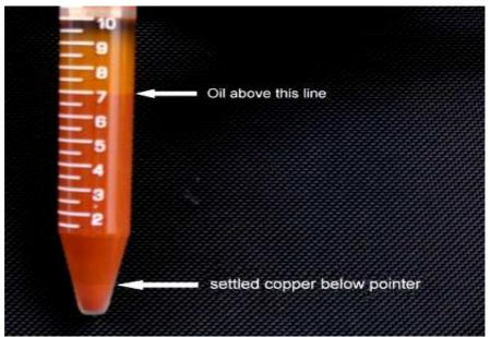
Figure 2. Three separated components of spray mixture.
