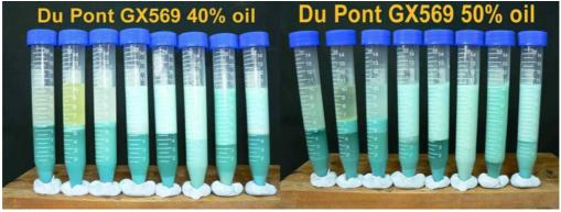
Figure 6a & 6b. Du Pont, GX569 Copper hydroxide stability in 40% and 50% oil after 24 hours.
