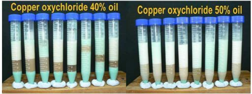
Figure 4a & 4b. Copper oxychloride stability in 40% and 50% oil after 24 hours.
