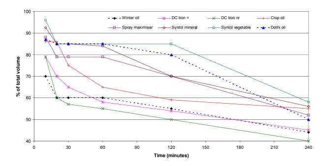
Figure 7. Cuprous oxide stability test for eight different spray oils over time.
