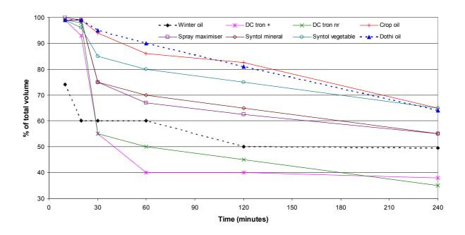
Figure 9. Kocide stability test for eight different spray oils over time.
