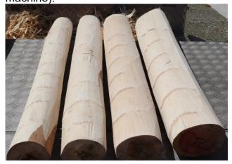
On the logs that had not been de-darker prior to post production it was found that the bark could be successfully removed from the *E. bosistoana and E. quadrangulata* (sometimes two passes through the machine were needed) with the Posch machine but the thick bark on the *E. globoidea* did causes issues such as blocking the machine and required frequently cleaning (photo below shows the *E. globoidea* after one pas thorough the Posch machine).
