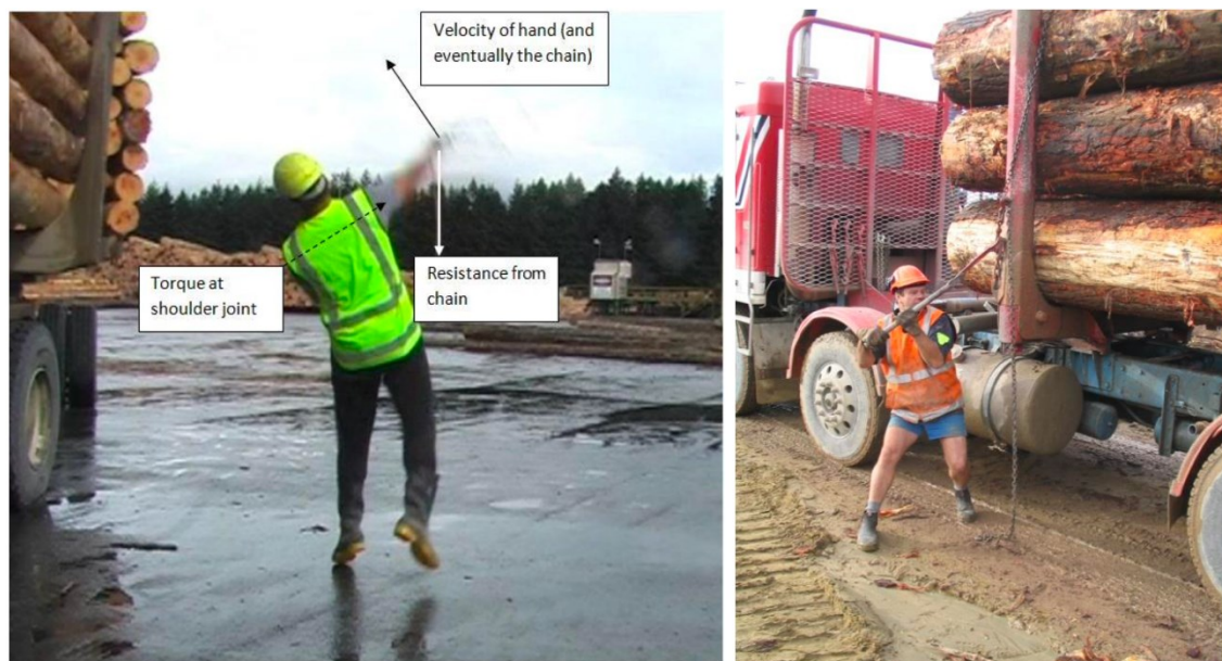
Figure 1. Forces involved in chain throwing and twitching to secure log loads (LTSC, 2020)
