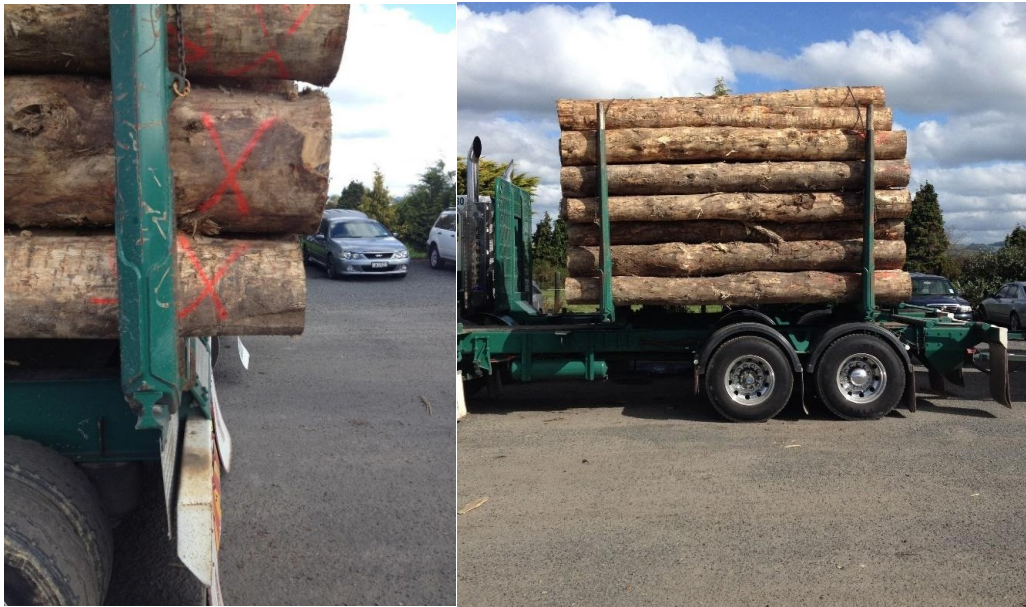
Figure 2. Photos of overhang required when loading 3.1m logs Source: David Adams
