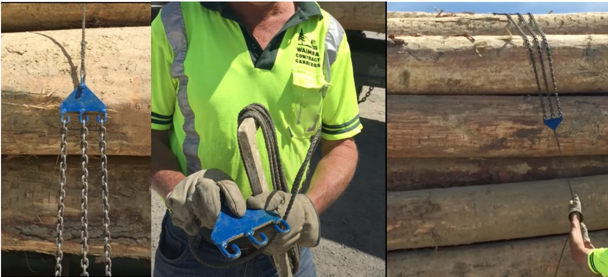
Figure 13. The triangle Hook and Throw Rope developed by Grant Soper
