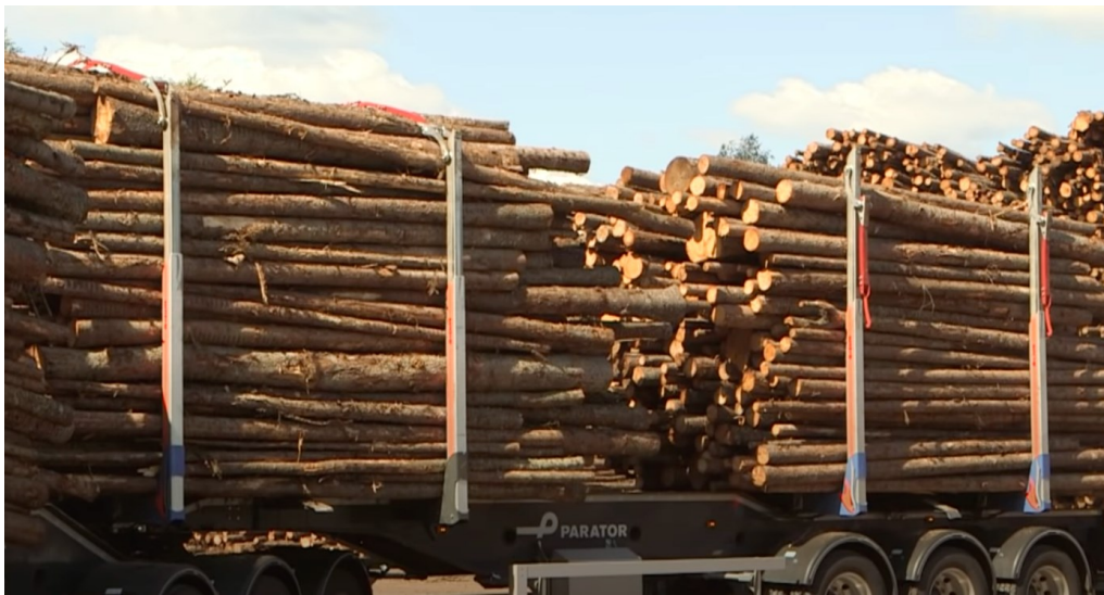
Figure 14. ExTe's Com90's automatic log securement. Source:
