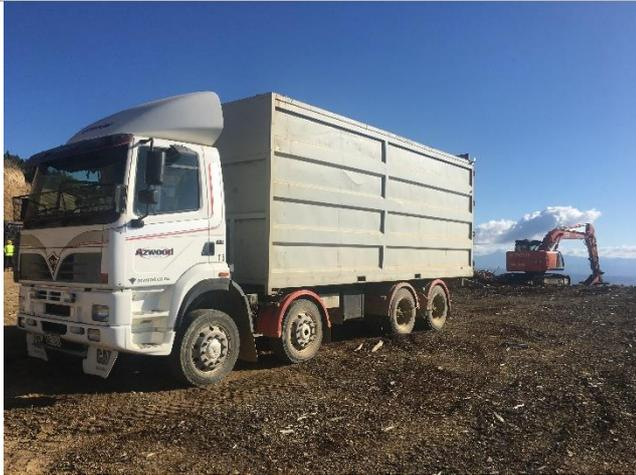
**Figure 8: Post-harvest recovery using the excavator and bin wood truck.**
