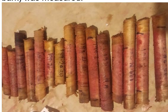
Figure 1: E. globoidea cores with heartwood dyed pink after application of methyl orange.
