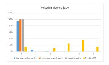
For the stake tests, some euc samples have failed, and the remaining stakes have well established to deep and severe decay. See figure below – all the eucalypt data has been combined to one column.
