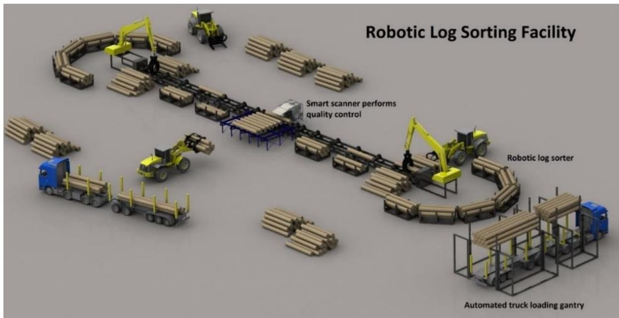
Fig 2: Proposed robotic log sorting facility
