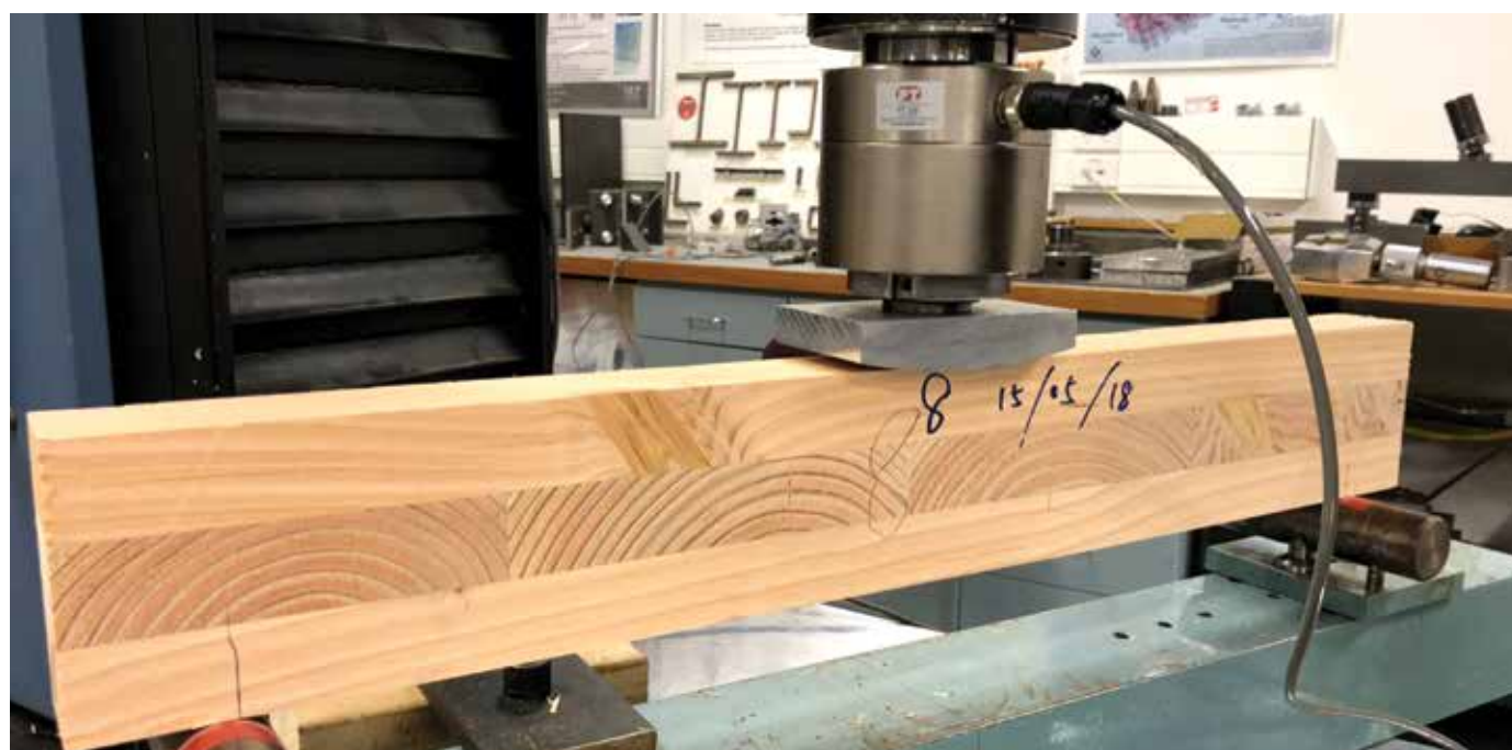
Figure 7: Strength testing of Douglas-fir CLT element
