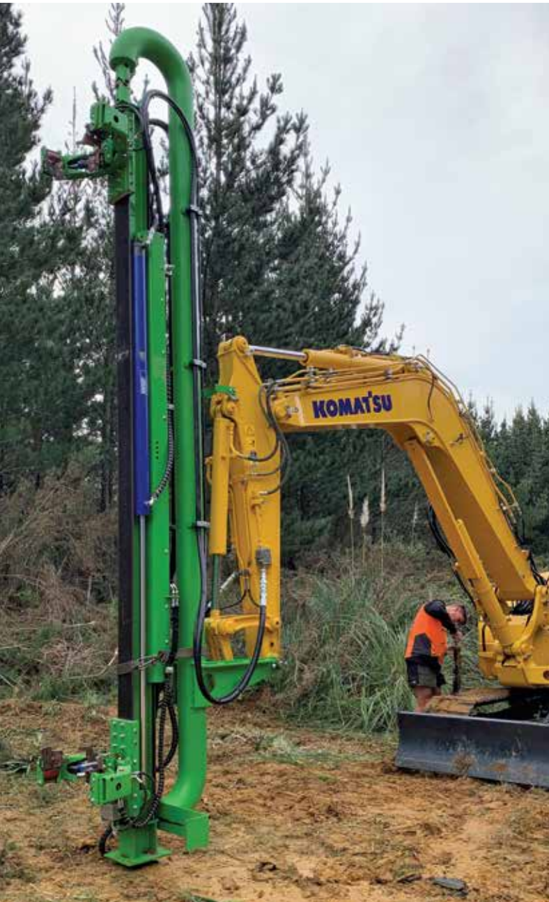
Figure 8: Hudson Clearwood pruning machine undergoing field trials
