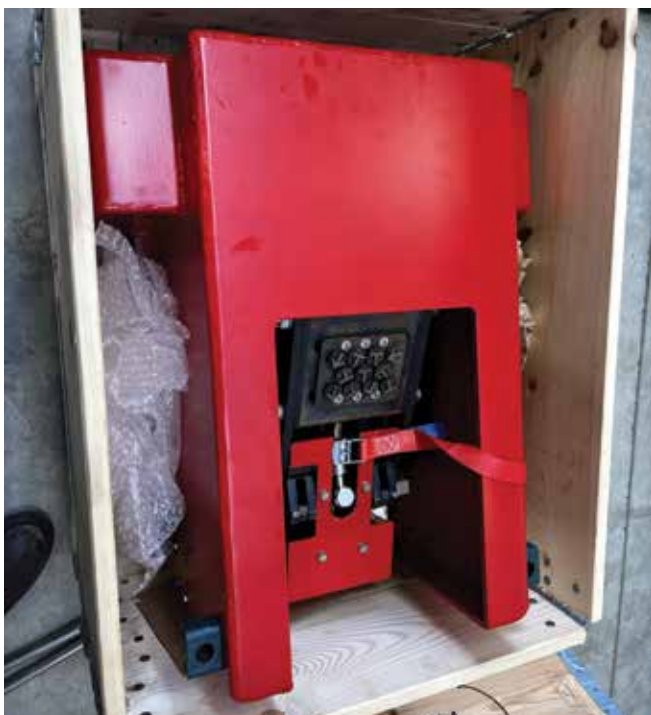
Figure 3: Otmetka log marker prototype ready for installation on Woodsman processor
