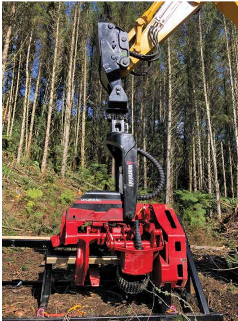
Figure 4: Steelwrist SQ80 coupler with Waratah 624 processor attached (note processor cradle)
