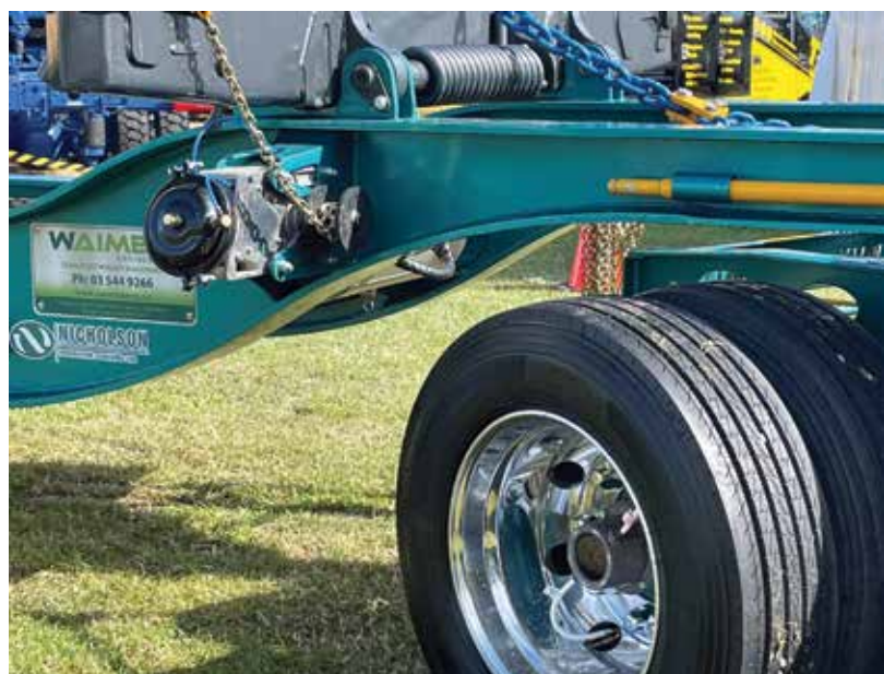
Figure 5: Trinder Engineering auto tensioner mounted on a log trailer
