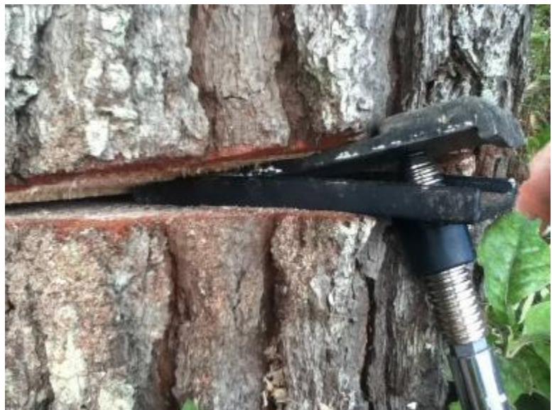
Figure 8: Flex in the plates and slot cut out for insertion
