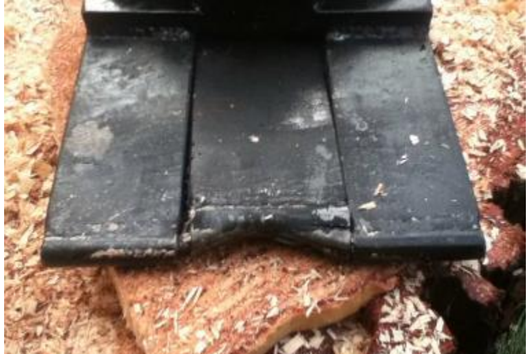
Figure 15: Bent hinge pin on the Wedge
