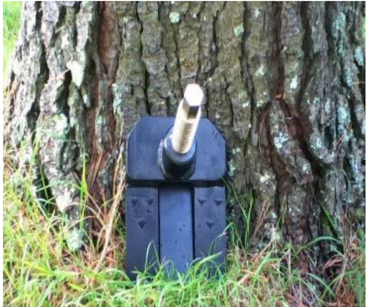
Figure 17: Final Wedge Design showing grip teeth
