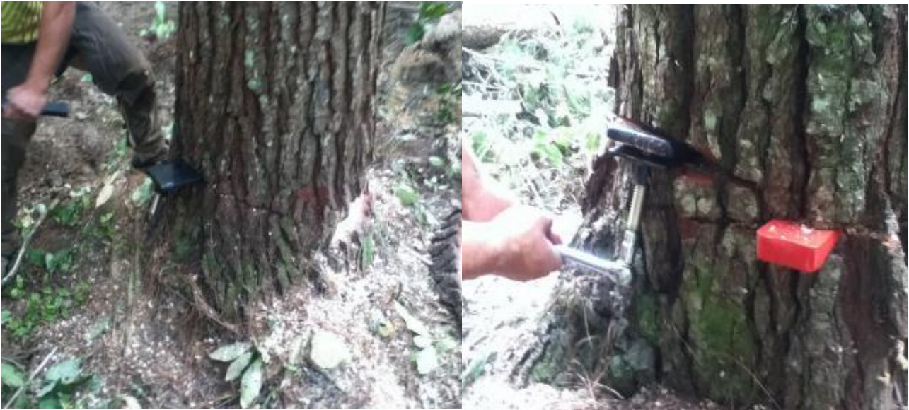
Figure 9: Using the hammer to drive in the wedge (left) and used with a conventional wedge (right)
