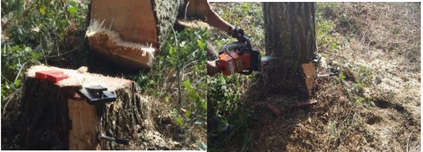
Figure 11: Bark cleaned and slot opened in the back cut for full Wedge insertion (left) and Wedge lifting trees over successfully with conventional wedges (right)
