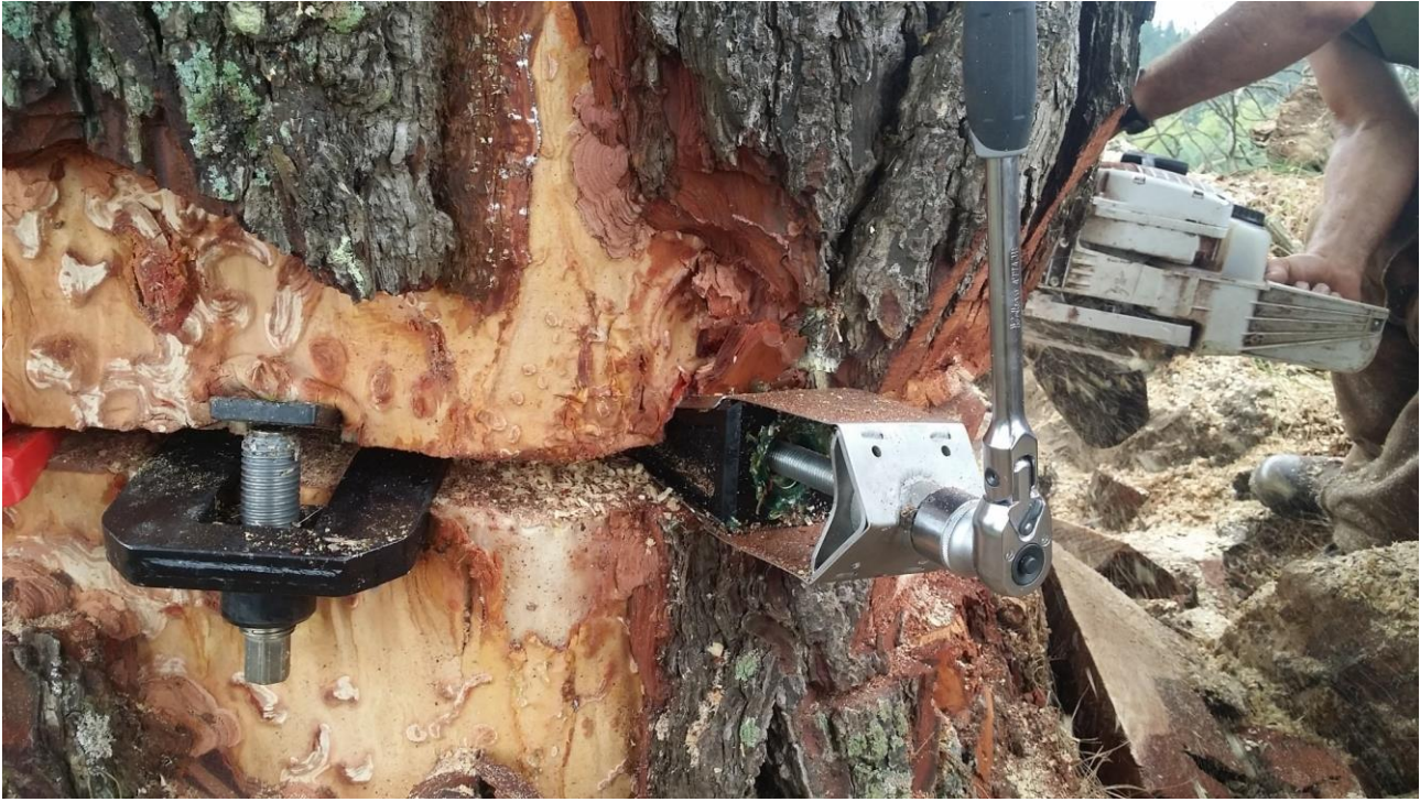
Figure 3: The JBL Wedge (left) and Koller Wedge (right) working together
