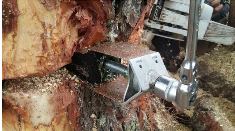
Figure 5: Universal joint on the ratchet handle of the Koller wedge
