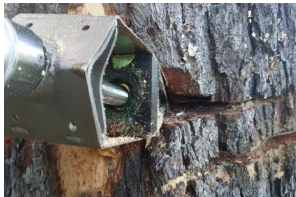
Figure 14: Koller pin screw going beyond the maximum line
