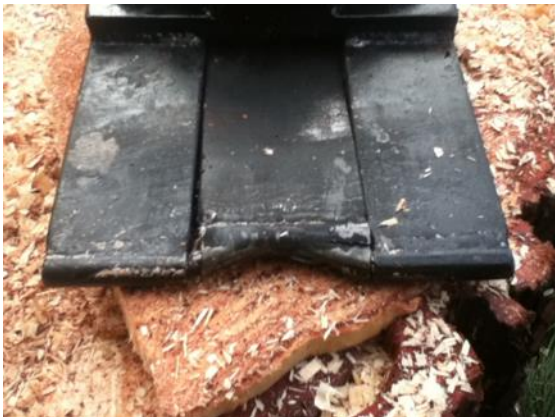
Figure 17: JBL bent hinge pin
