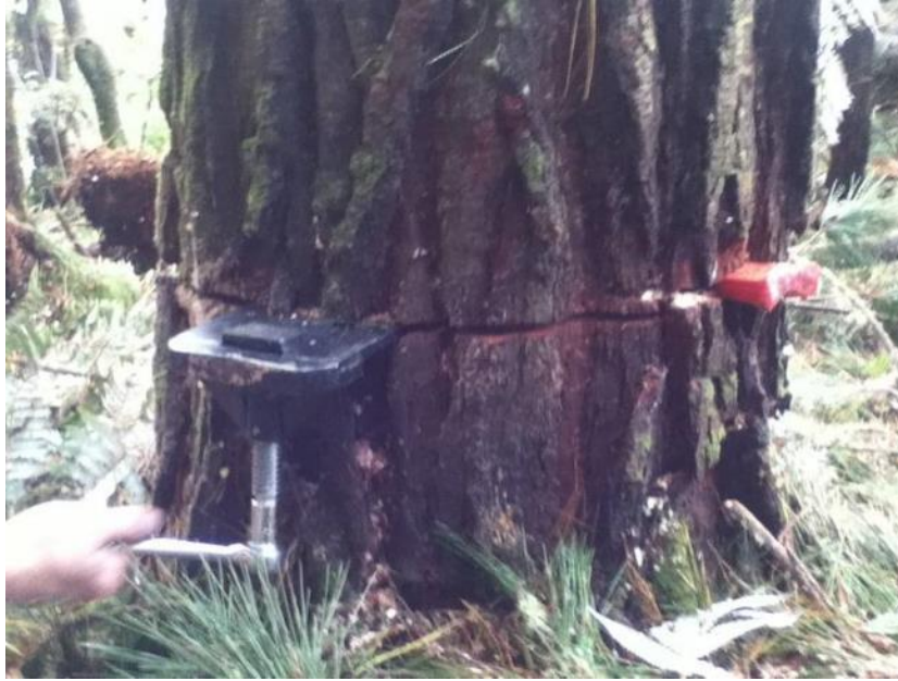
Figure 1: The prototype Jackson Beckham Felling Wedge
