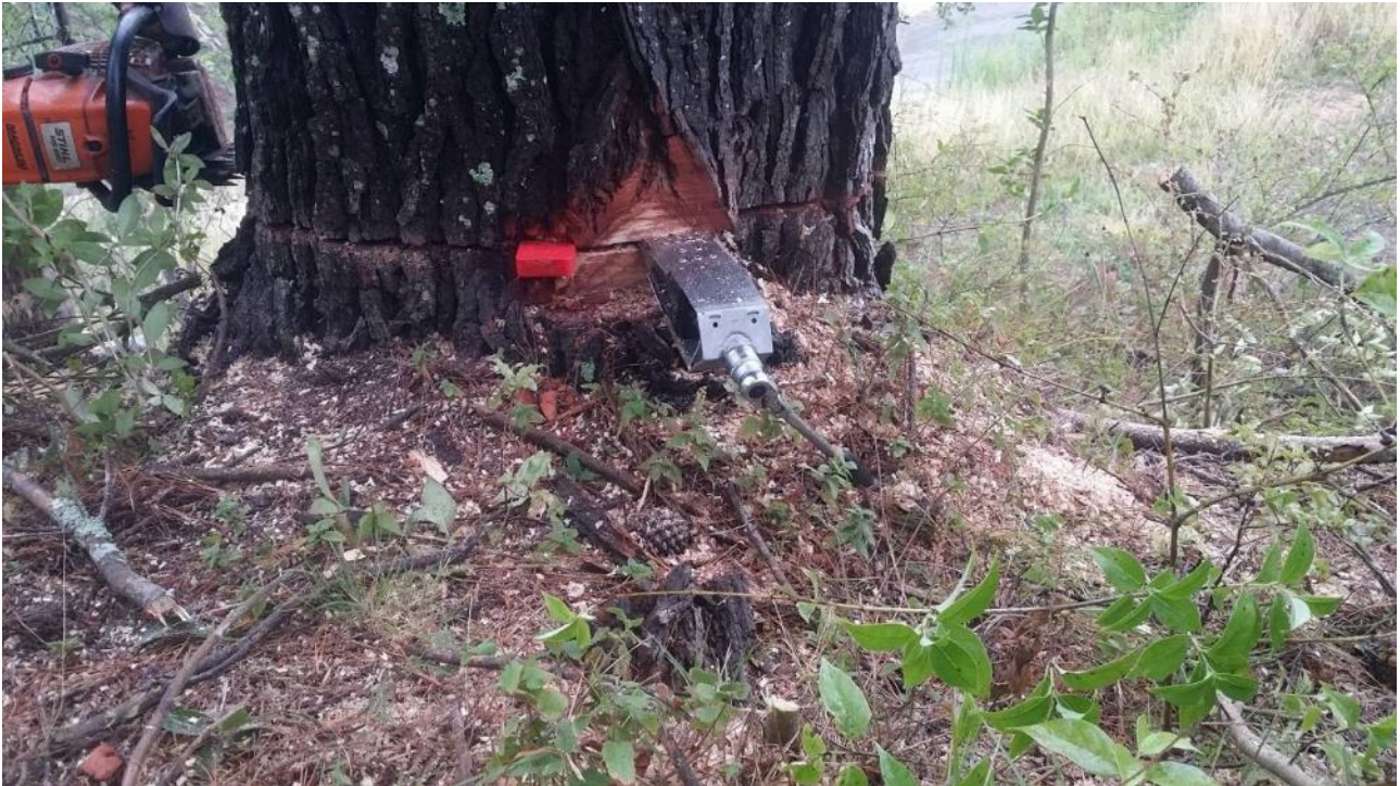
Figure 4: Koller wedge in action in Waitotahi Valley Forest
