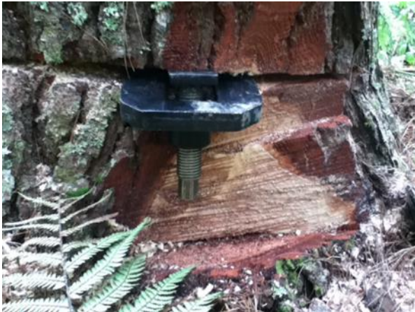
Figures 15: JBL top plate pushing into the tree
