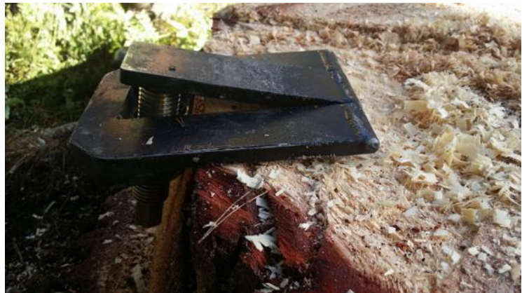
Figures 9 and 10: JBL wedge insertion depth
