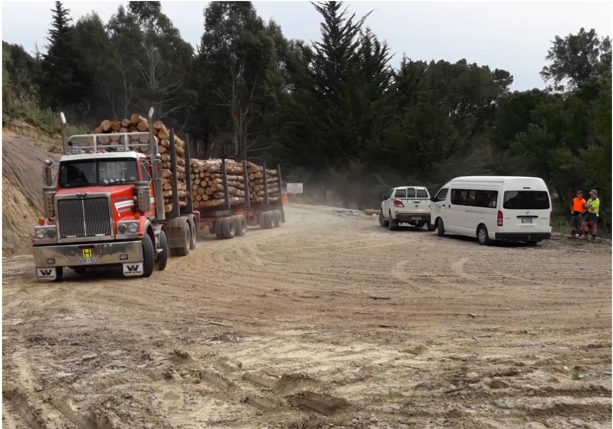
Figure 1. An 8-axle truck and trailer combination traversing a switchback on a steep forest road in Canterbury.
