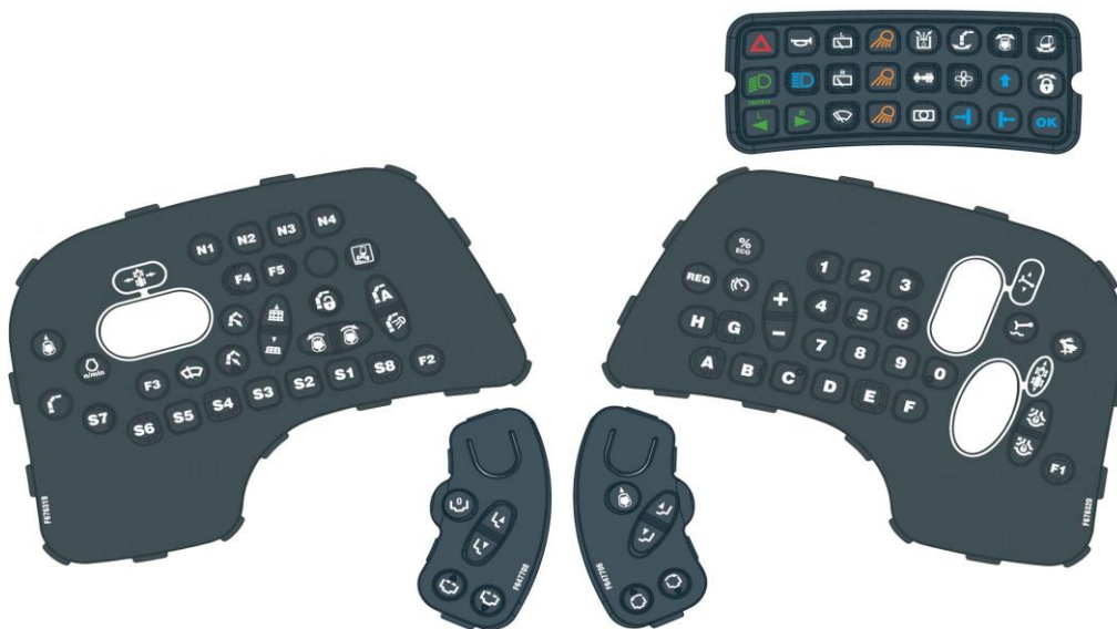
Figure 2: Basic control layout for John Deere forest machine simulator.
