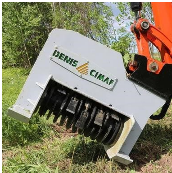
Figure 13. Denis Cimaf mulching attachment from the DAH boom-mounted mulcher series. Source: https://www.morbark.com/products/mulching-attachments/
