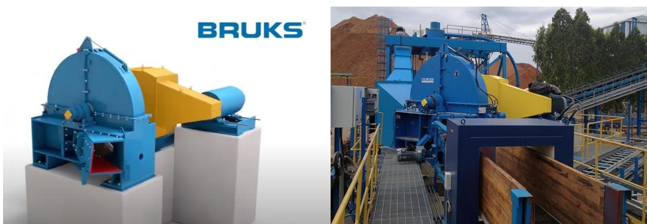
Figure 14. The Bruks siwertell horizontal fed disc chipper.
